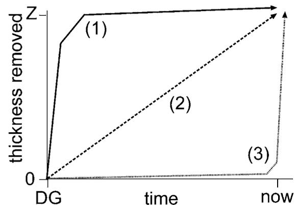
**Fig. 2.** Scenarios used to correct cosmogenic ages for subaerial erosion.  $Z$  = total erosion thickness, indicated by height difference between sampled surfaces and striated surfaces nearby, DG = deglaciation. (1–3) mark scenarios as described in text.
