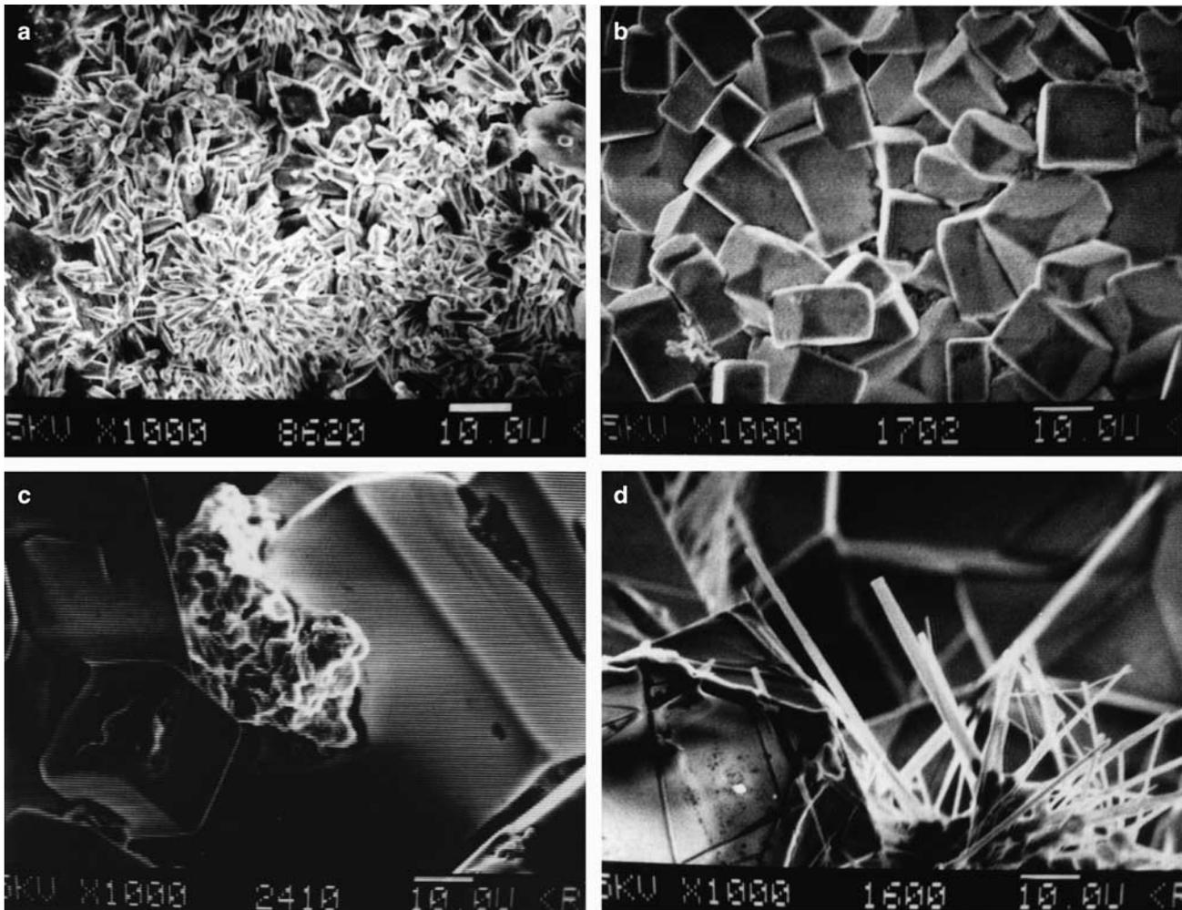
**Fig. 4.** Representative salt minerals. **a.** Top left: flowers of gypsum ( $\text{CaSO}_4 \cdot 2\text{H}_2\text{O}$ ). **b.** Top right: cubic crystals of halite ( $\text{NaCl}$ ). **c.** Bottom left: amorphous gypsum nestled between cubic halite crystals. **d.** Bottom right: acicular thenardite ( $\text{Na}_2\text{SO}_4$ ) with cubic halite. These samples are from Broknes, and the scale bar on each photomicrograph is  $10 \mu\text{m}$ .
